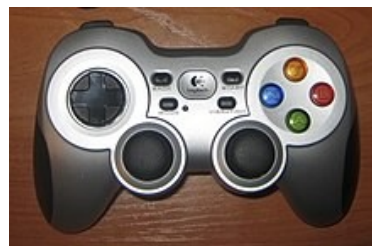
Logitech F710 wireless game controller was modified to serve as the thrust controller.
